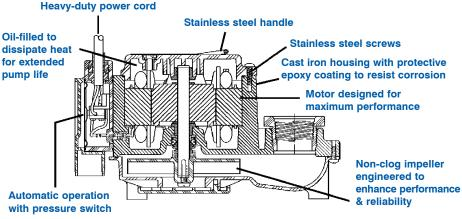
For residential and light commercial use, the Model 6-CIA sump pumps provide efficient and reliable service. For extended or continuous use in moving large volumes of water, these pumps feature a 1-1/2" discharge with a maximum lift of 18', a polycarbonate cover and a polypropylene volute/base.
