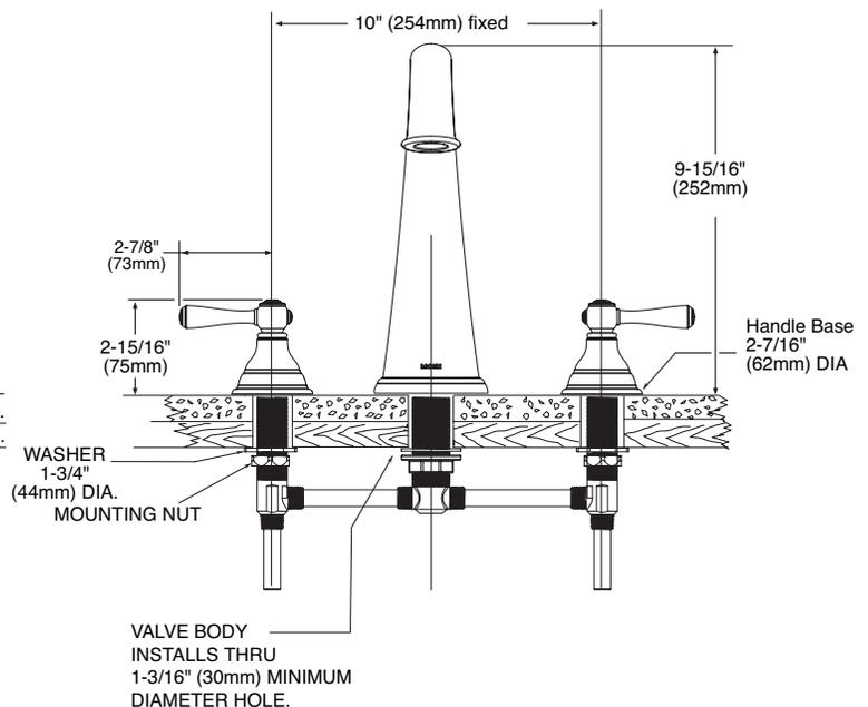
**NOTE: THE INSTALLATION SHOWN IS FOR TILE DECKS, THIS VALVE WILL ALSO FIT STEEL, CAST IRON OR PLASTIC DECKS**
